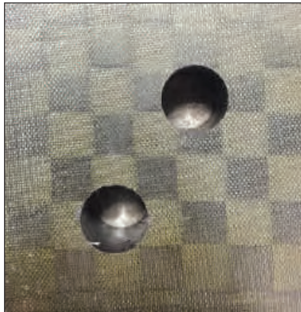
Holes drilled with PCD tooling
