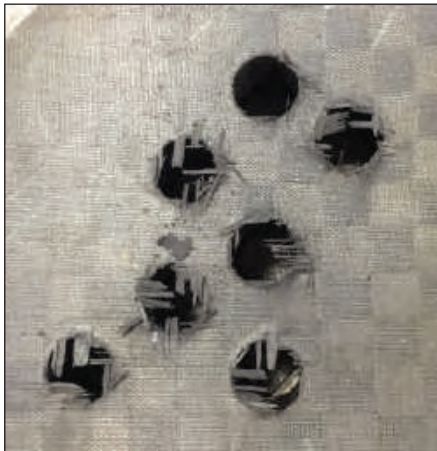
Holes drilled with CVD drill insert
